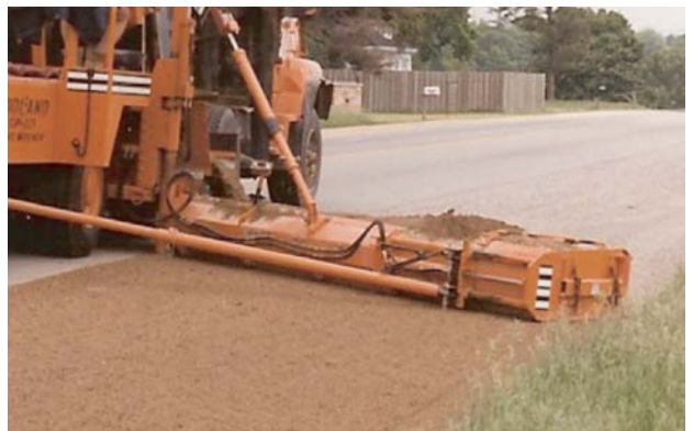
Modular blade sections and a 2-4 ft hydraulic extension
