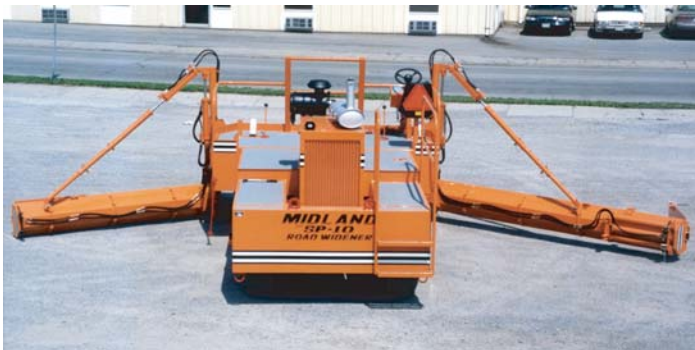
Quick change from right to left discharge
