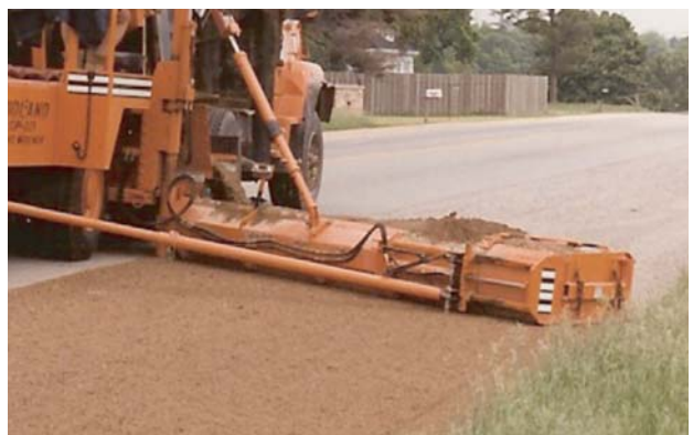
Modular blade sections and a 2-4 ft hydraulic extension
